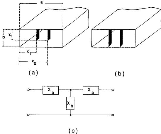
Fig. 1. Geometry of the E-plane (a) nontouching and (b) touching bilateral septum in waveguide. (c) Its corresponding T-equivalent circuit.
