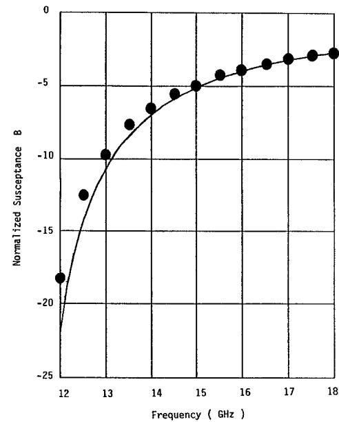
Fig. 2. Normalized input susceptance of the bilateral septum in Ku-band waveguide with  $a = 16.12$  mm,  $b = 8.10$  mm,  $x_1 = 6.497$  mm,  $x_2 = 9.623$  mm, and  $w = 0.5$  mm. (a) Nontouching case with  $y_1 = 6.51$  mm. (b) Touching case with  $y_1 = 8.10$  mm. — Computed data using this technique. ● ● ● Measured data.
